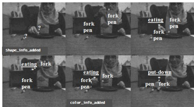
Fig. 9. Recognition results of a fork and a pen where both have the same shape. Results of the object recognition algorithm are given as labels embedded on to each frame of the video. Video is taken from the left-eye camera of a QRIO robot.
